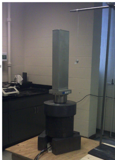
Fig. 4. Experiment setup of Heath (left) and rectangular NaI detector at CEAR (right).
